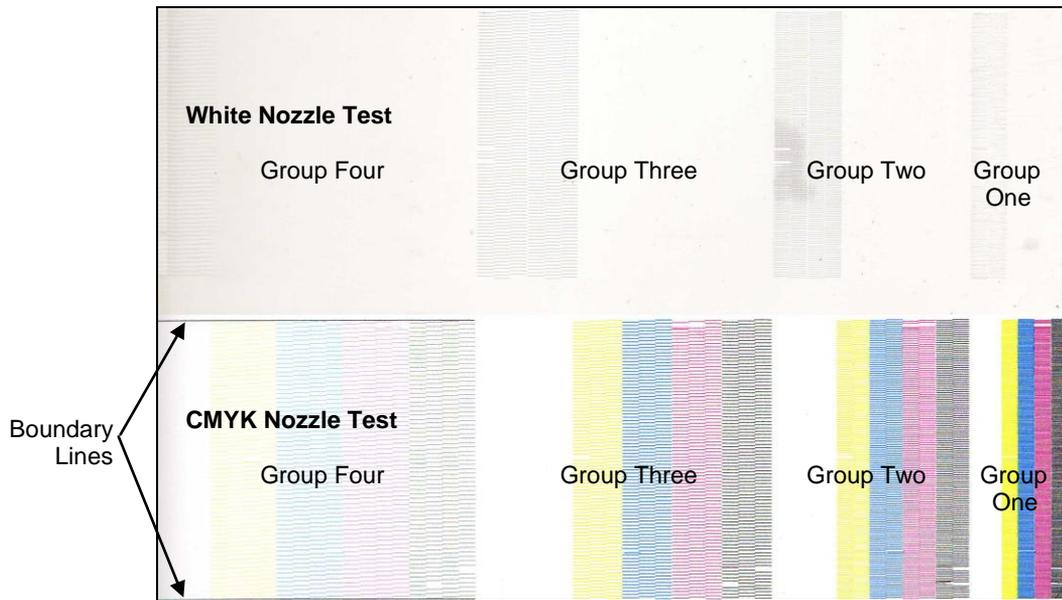
Figure 48: Nozzle Test Image
