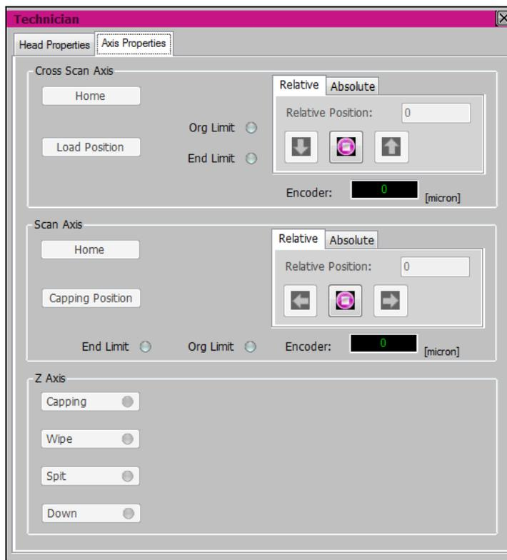
Figure 29: Technician Window/Axis Properties
