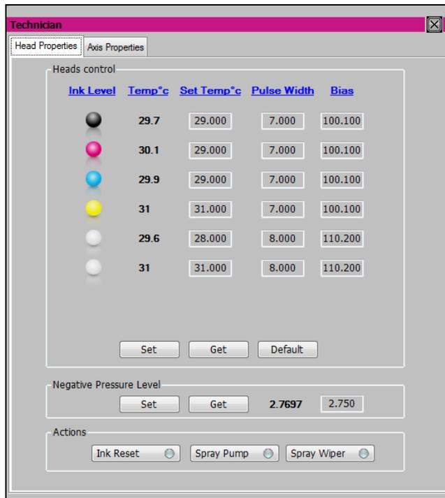
Figure 28: Technician/Head Properties Window
