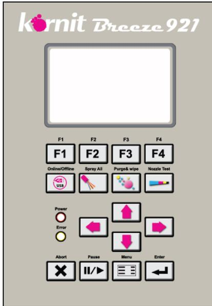
Figure 128: LCD Maintenance Panel
