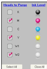
Figure 133: Ink Valve Controls
