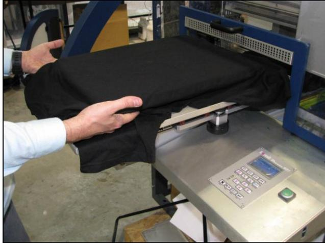
Figure 53: Folding Under Excess Garment
