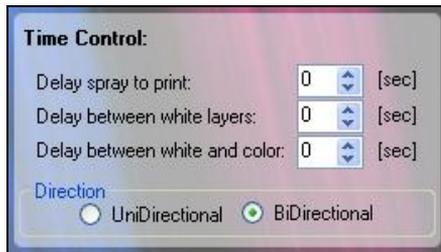
Figure 23: Time Control and Print Direction Panel
