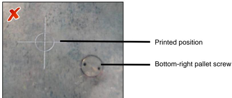
Figure 112: Incorrect Print Alignment
