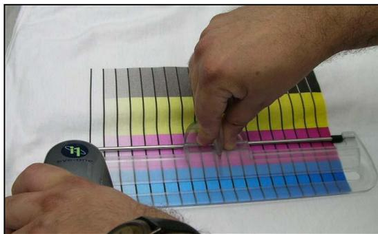
Figure 123: Pressing the Scan button
