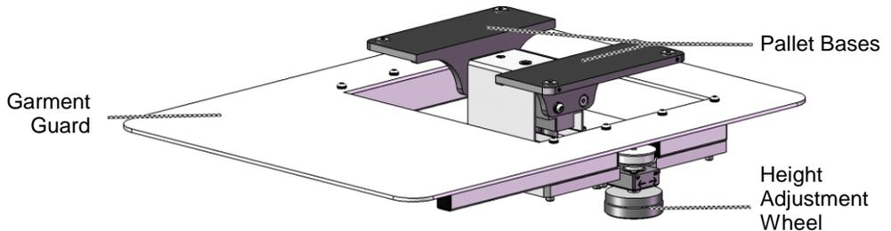
Figure 86: Height Adjustment System
