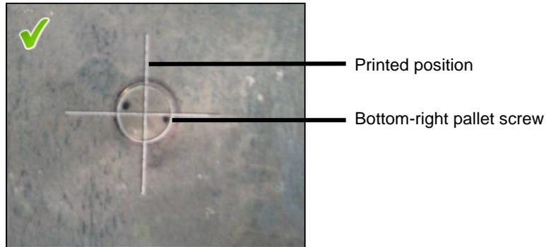
Figure 111: Correct Print Alignment
