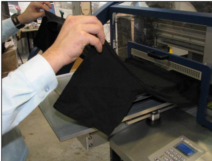
Figure 52: Placing the Garment
